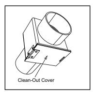
Figure 19.3 - Rear Vent Adapter
